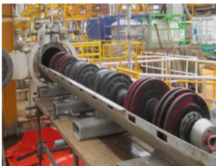
SmartPlug® tool retrieved after the 299-day isolation.
